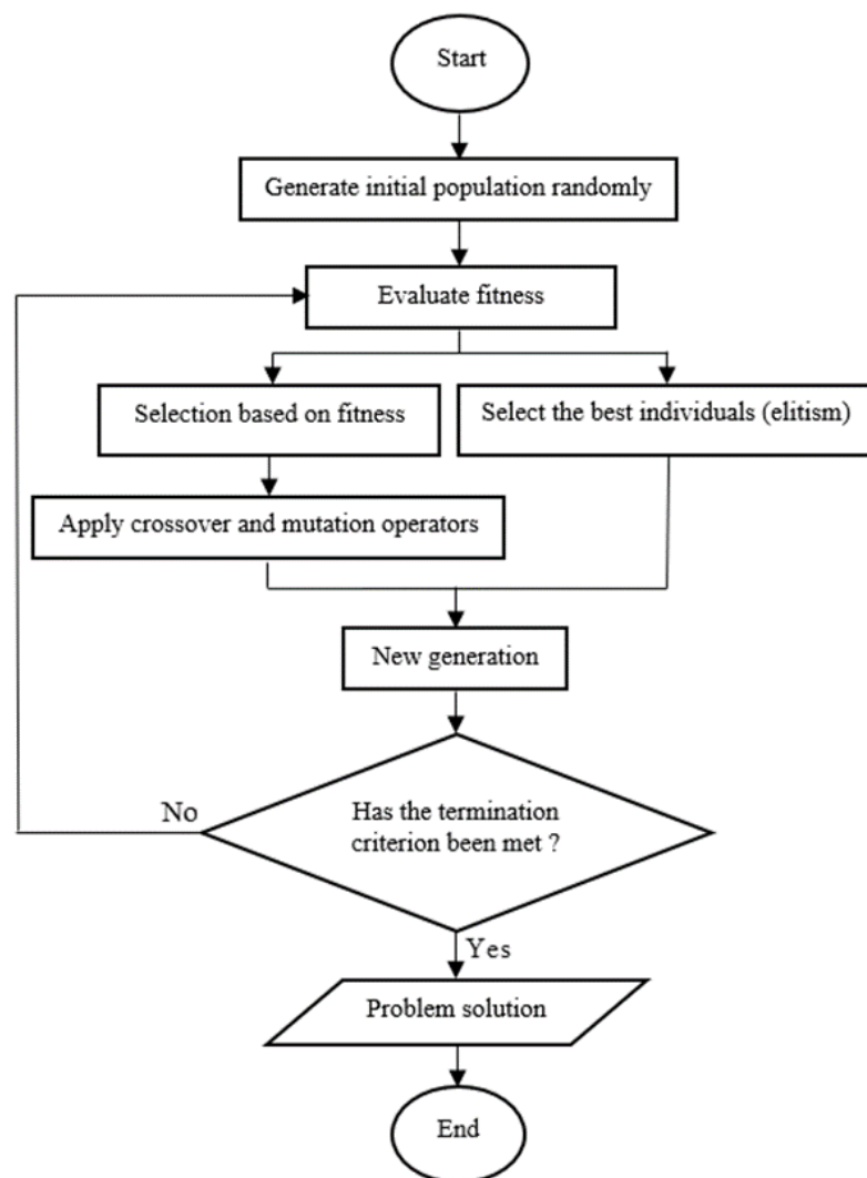
Figure 2: Flowchart of the Genetic Algorithm
