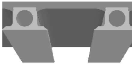
Figure 2. Slab section formed by unialveolar beam
