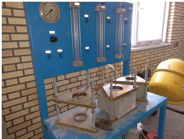
Figure 17 An image of the permeability test apparatus
