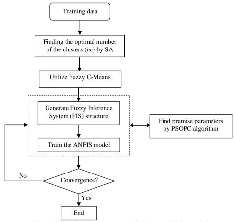
Figure 2. Flowchart of the proposed intelligent ANFIS model
