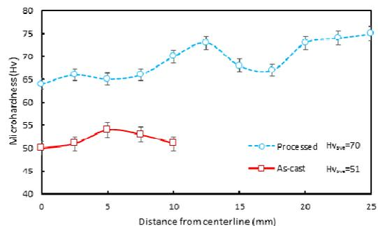
Fig. 5. Microhardness variations along with samples diameter
