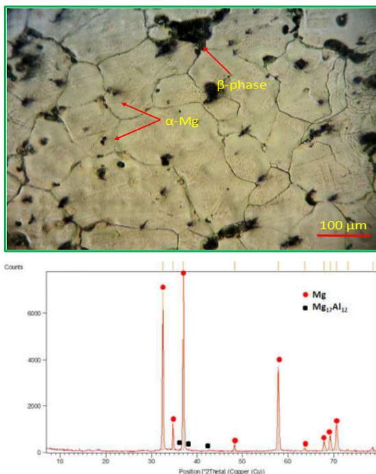
**Fig. 3.** The microstructure of the as-cast AM60 magnesium alloy with coarse grains of  $\alpha$ -Mg and intermetallic  $\beta$ -phase ( $\text{Mg}_{17}\text{Al}_{12}$ ), and corresponding XRD pattern.
