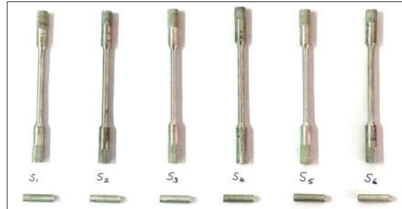
Fig. 3. Tensile and wear test samples
