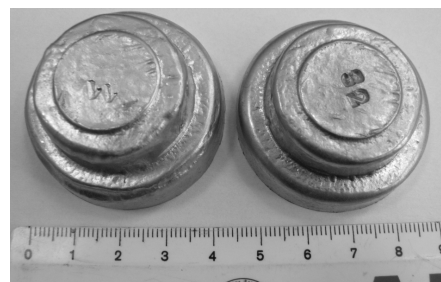
Fig. 1. Samples for testing the alloy porosity content
