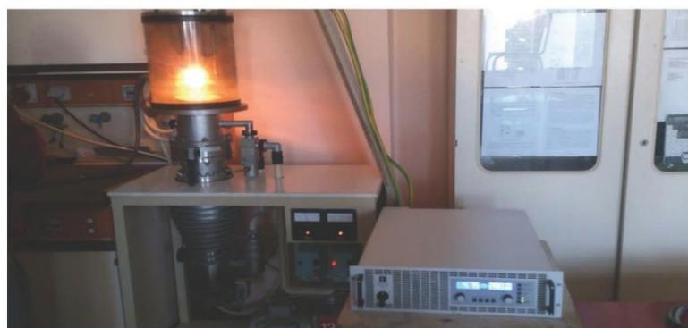
Fig. 1. Working evaporation chamber
