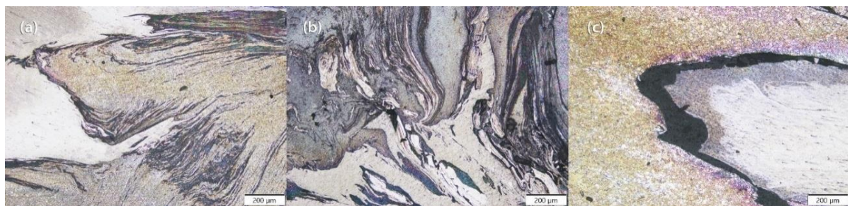
Fig. 15. Stir zone Microstructures for a) low b) middle and c) high parameter combinations
