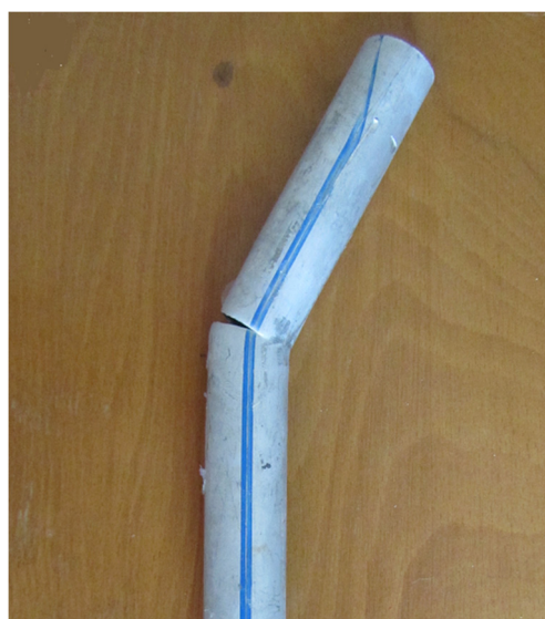
Fig. 10. Fractured AA 6063-T6 tube after (a) simulation and (b) experimental bending test at a bending radius of 32.5 mm.
