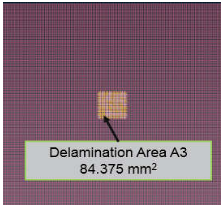
Fig. 3. Top view of delamination incorporated.
