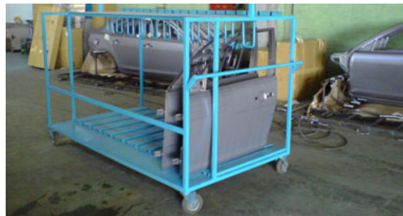
Fig. 1. Mobile material handling shelf
