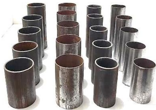
Figure 3: Experimental specimen sets of cylindrical tubes made of mild steel.
