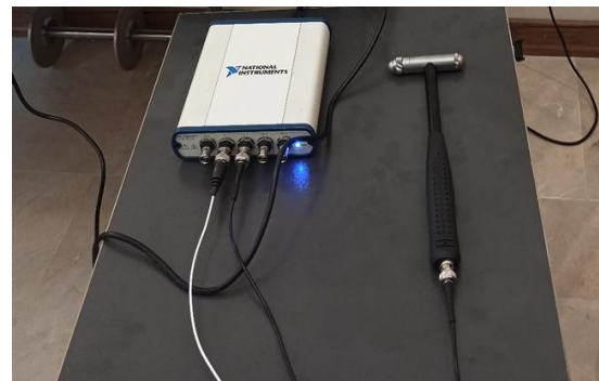
Figure 6: Data acquisition card and impact hammer used for modal analysis testing
