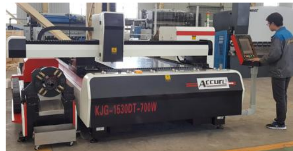
Figure 1: ACCURL laser tube cutting machine in operation
