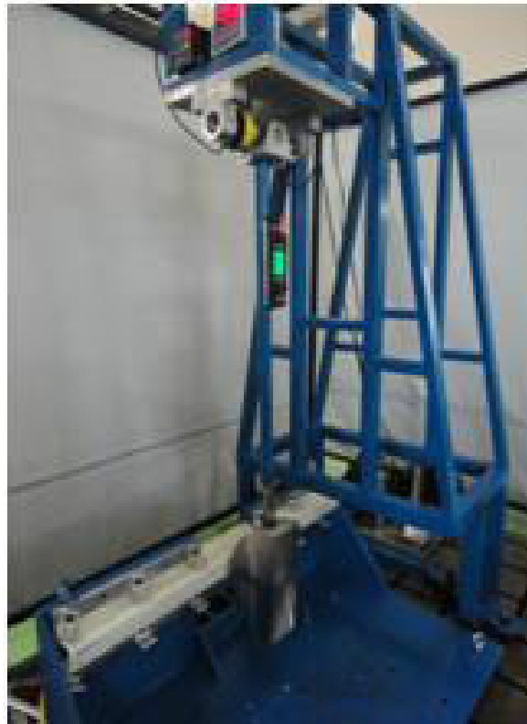
Fig. 5. Impact loading bending test machine
