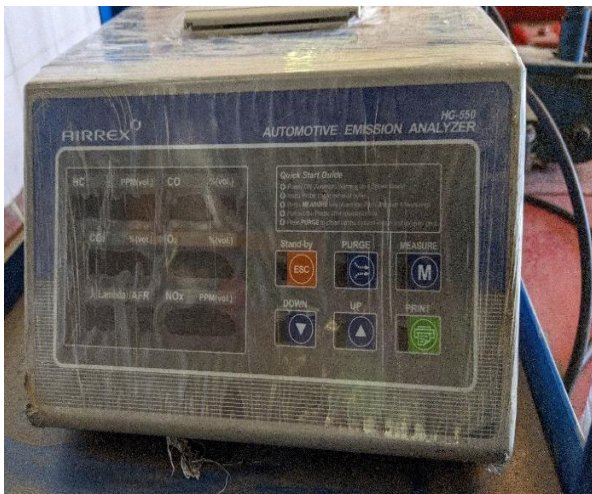
Figure 3: Exhaust gas analyzer
