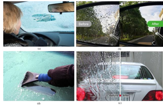
Figure 2: (a) Frost formation is one of the main challenges of cold region drivers. Effect of superhydrophobic coating on (b) rear-view mirror and (c) front windshield. (d) Mechanical defrosting is only suitable for when the car is in park mode.
