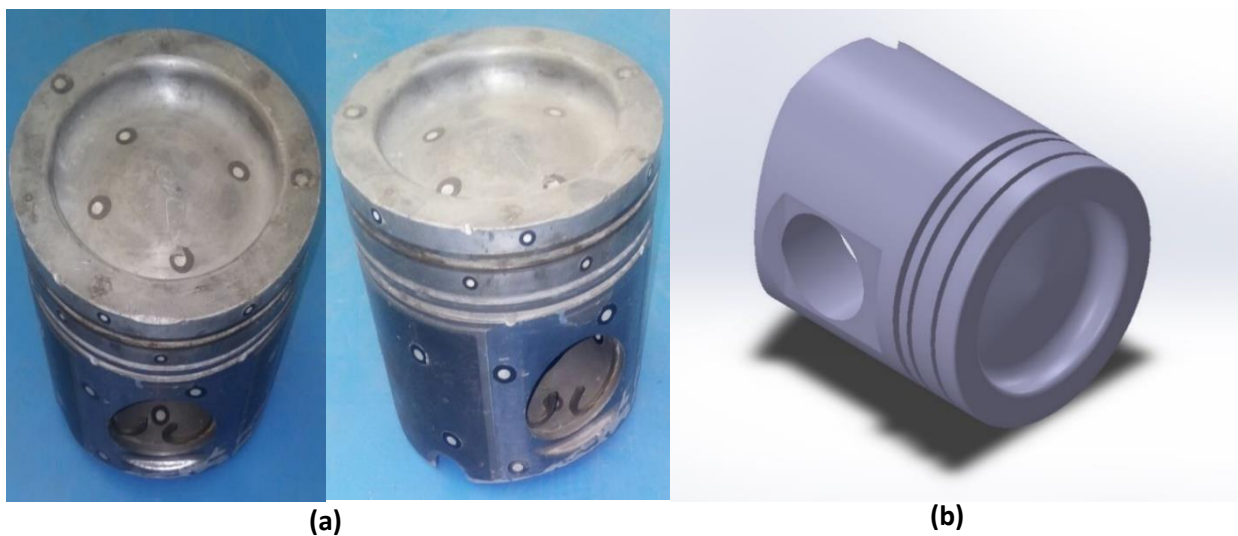
Figure 1: OM457's piston head a: real one – b: .stl file of OM457's piston head used for CFD analyses
