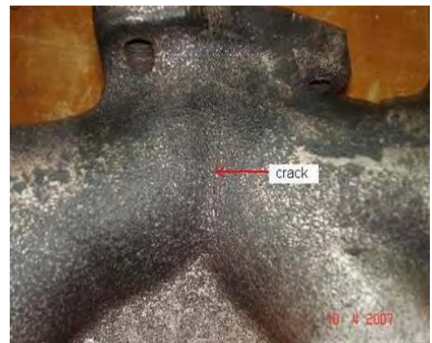
Figure 5: The cracked exhaust manifold
