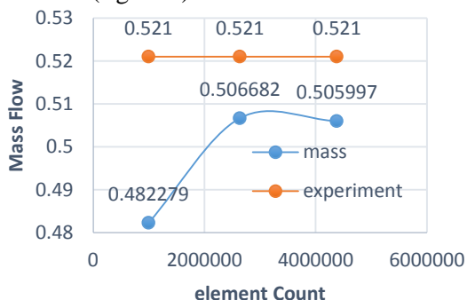
Figure 1. Mesh sensitivity analysis of whole turbine Both the full and the partial admission analysis used the same mesh.
