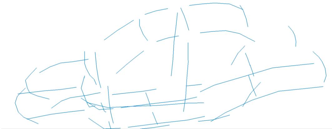
Fig3.: Equivalent beam modeling of the BIW
