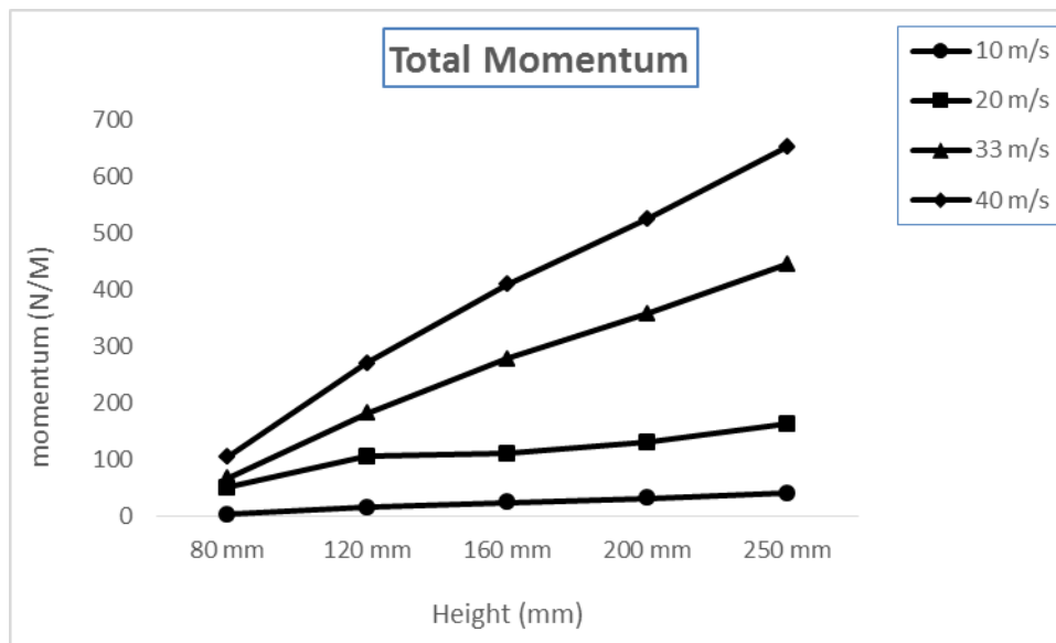
Fig.11. Changes in the torque around the automobile center of gravity
