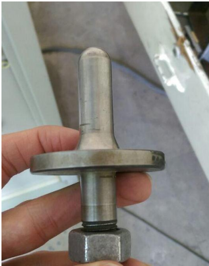
Fig2.Steel imp actor used in drop ball tests
