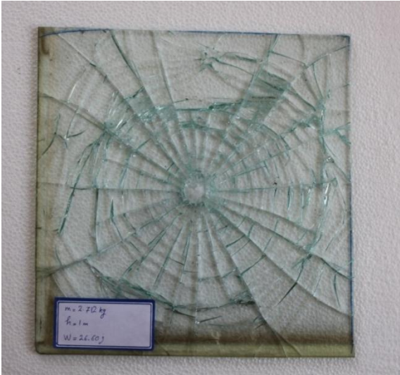
Fig14. .specimen after test code D-B-T-6
