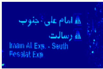
Fig11. Stroke Width Transform of the image.
