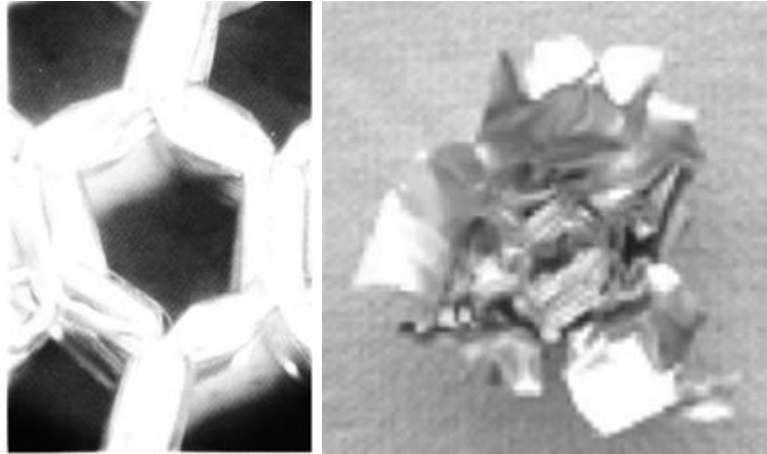
Fig3. (a) Crushed aluminum honeycomb core near the penetrated region (b)Produced plug from aluminum honeycomb core at 94 m/s impact velocity
