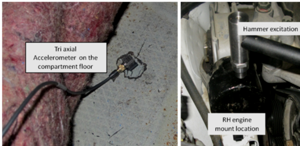
Fig6. Body transfer function measurement of RH mount: excitation point and accelerometer
