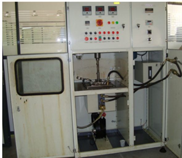
Fig16. Test setup of external gear pump
