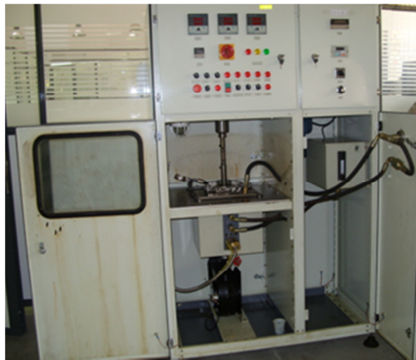
Fig16. Test setup of external gear pump
