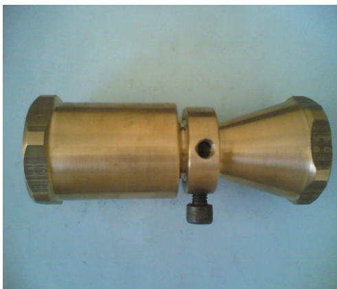
Fig. 13. Schematic of optimum venturi
