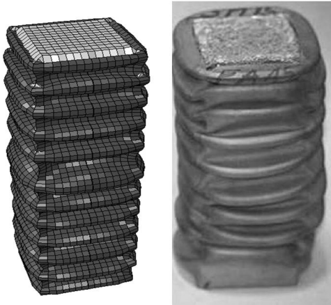
Fig5.. Comparison of experimental deformation [22] with numerical prediction.
