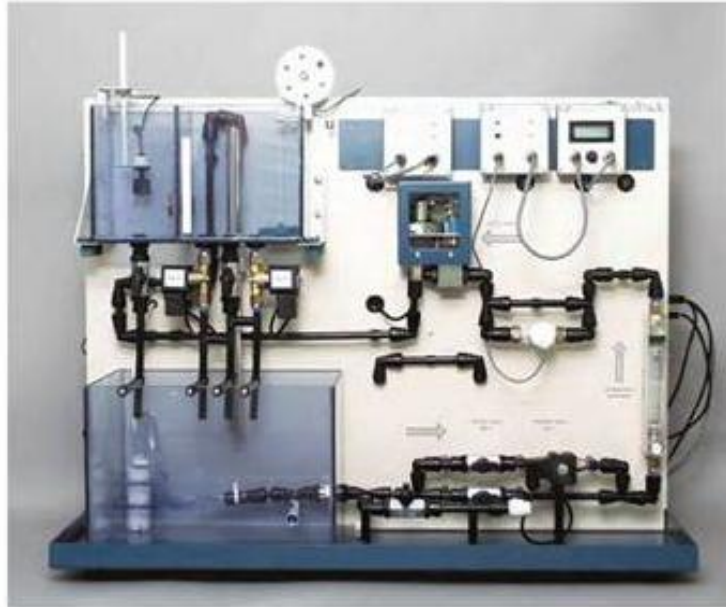
Figure 1-9: Level and Flow Process Rig
